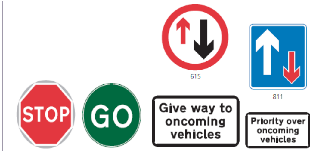
Figure 1.4: Manually operated stop/go signs and priority signs
